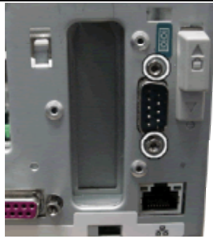
Fig. 19: Removing the second serial port
